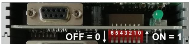
Figure 16 – Switch for setting the slave address with back plate removed
